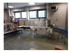
Forming both single and twin wall cases for Hobbs, the 221, has a maximum speed of 18 cases per minute.
