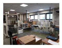
From the gravity roller conveyor, manual operators take the formed cases, placing them on packing tables for filling. The two packing tables, which Endoline installed for ease of operator movement, are positioned either side of a powered roller conveyor.
